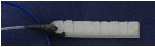
Fig. 8: The assembled fabricated soft pneumatic actuator.
